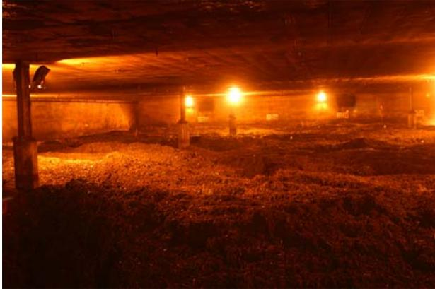
Blended feedstocks are placed into compost piles over air grates that pull air through the pile to control temperatures and supply oxygen to the microbes.
