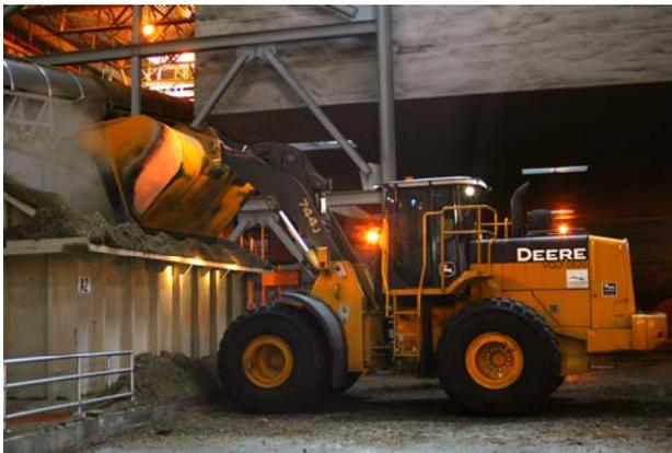
Woody amendments are loaded into hoppers prior to mixing with the biosolids.
