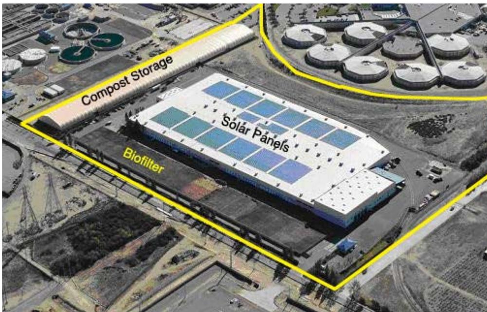
On the roof of the Inland Empire Regional Composting Facility are over 6,000 solar panels that can produce up to 1 megawatt of electricity. The biofilter occupies over 3 acres at the lower portion of the photograph. To the left is a compost storage facility, able to hold up to 3 months' production as needed in winter, when sales typically slow.
