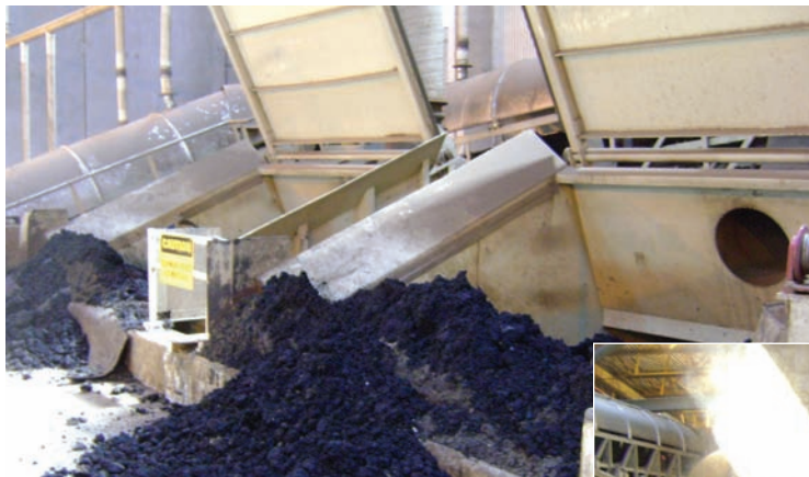
Biosolids are tipped directly into designated hoppers (left). Bulking agents are blended and scooped into an amendment hopper with a front-end loader (below). The hoppers feed materials onto a conveyor that leads to pug mill mixers.
