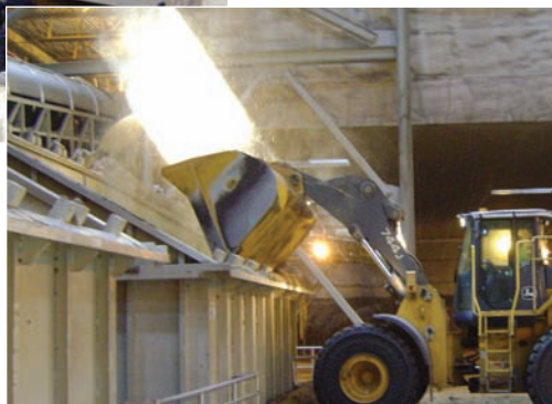
Biosolids are tipped directly into designated hoppers (left). Bulking agents are blended and scooped into an amendment hopper with a front-end loader (below). The hoppers feed materials onto a conveyor that leads to pug mill mixers.
